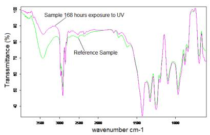
Figure 2. FTIR spectrums of reference sample and samples exposed to UV up to 168 hours.
