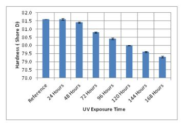
Figure 5. Hardness of sample with exposure time of UV.
