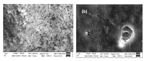
Figure 1. SEM images of (a) reference sample (b) after exposing to UV for 168 hours.
