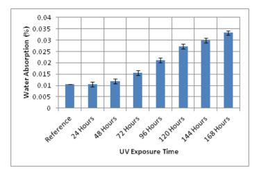
Figure 6. Water absorption of sample with exposure time of UV.
