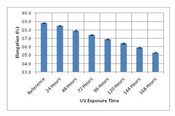
Figure 4. Relative elongation of sample with exposure time of UV.
