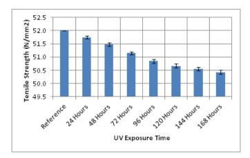
Figure 3. Tensile strength of reference sample and variation with exposure time UV.
